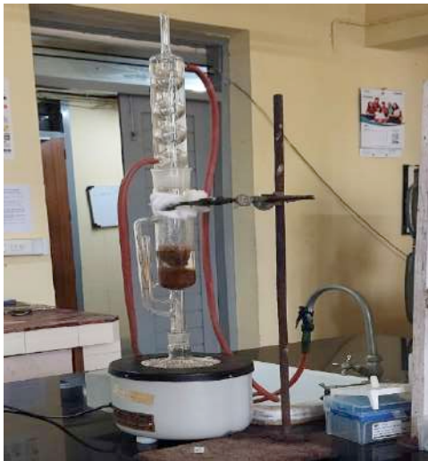
Figure 8: Soxhlet extraction of Pomegranate dried powder to obtain the bioactive extract
