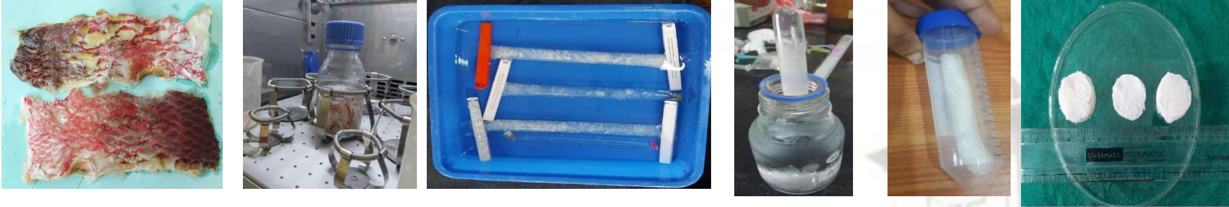
Figure 26: Different steps of fish collagen isolation from fish skin waste
