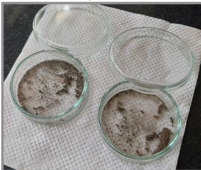
Figure 18: Synthesized by green synthesis method using Plant extract and Silver nitrate solutions- Phyto based silver nanoparticles
