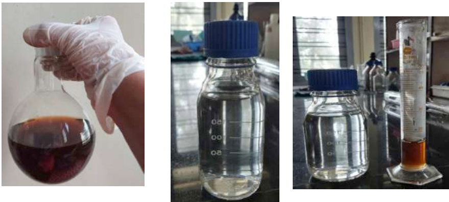
Figure 16: Synthesis of nanoparticles by green synthesis method, mixing of plant extract and silver nitrate solution and kept for hours to synthesize nanoparticles
