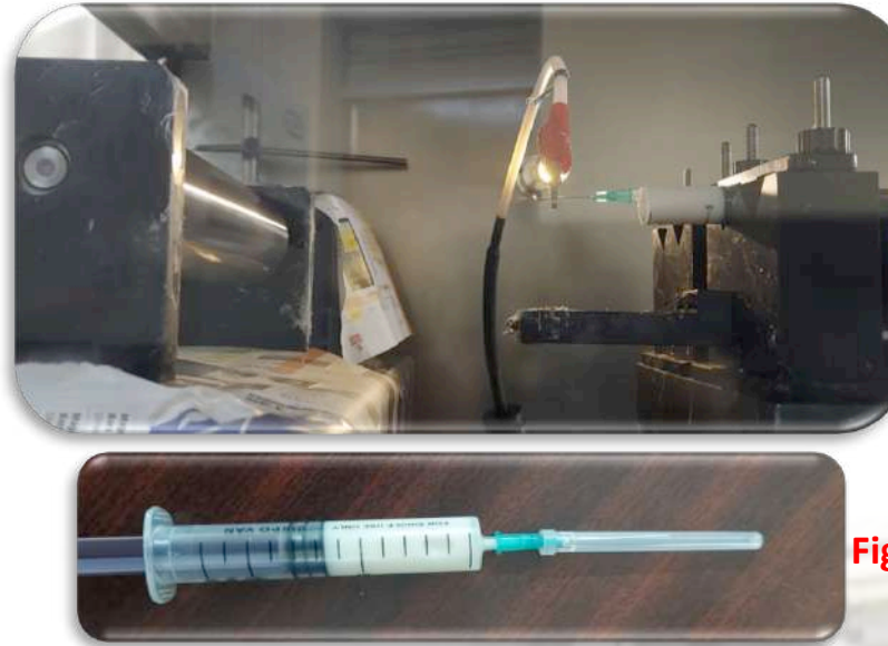
Figure 28: Electrospinning apparatus under the wound dress making process
