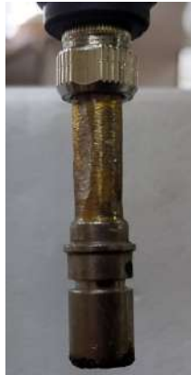
Figure 51: Burn creation apparatus
